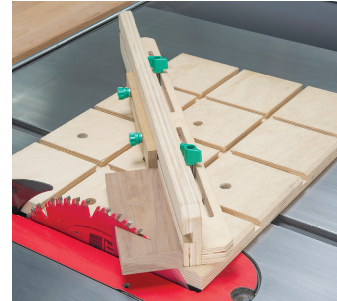
The unique grid layout of dovetail tracks allows the fence 360 degrees of rotation.
