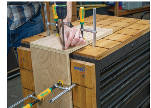
MATCHFIT Dovetail Clamps are a perfect space-saving solution. Just route dovetail tracks in your existing work surface, tool chest, or even sawhorses.
