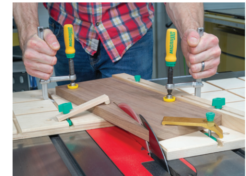
With the included, specially designed 1/2" 14-degree dovetail router bit, you can route your own tracks for jigs and fixtures, eliminating the need for expensive aluminum tracks.
