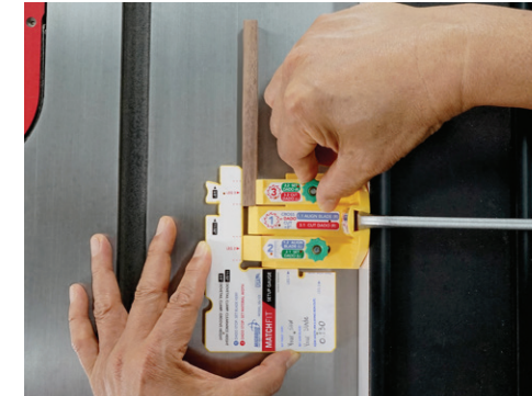
Set the legs of the Dado Stop to cut dados with any standard blade.
