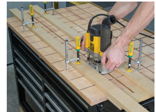
Route dovetail tracks into a table top to get even clamping pressure.
