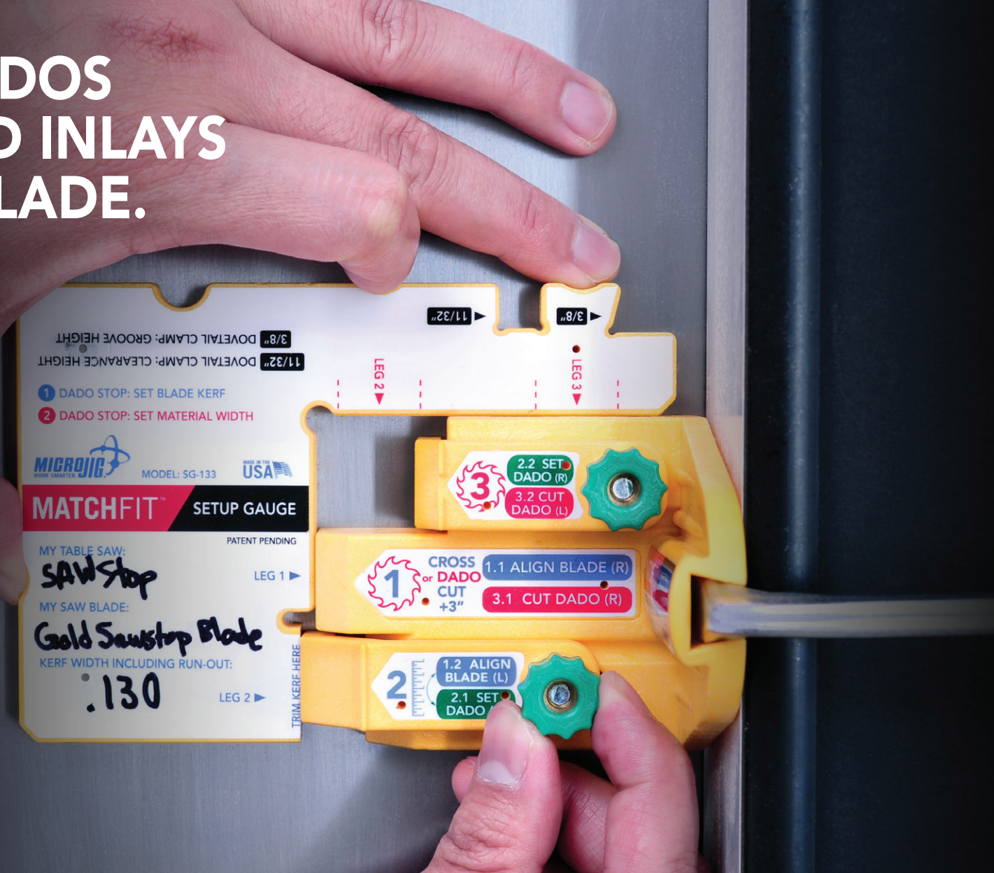
Set the legs of the Dado Stop to cut dados with any standard blade.
